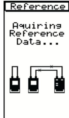
Once the reference value is established, consistent readings for loss, delay, and length measurements are ensured.
