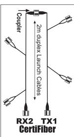
4. Remove the coupler without disturbing the connection to Certifiber.
